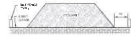
A STOCKPILE DETAIL, TYP. SCALE: N.P.S. SILT FENCE TO EXTEND AROUND ENTIRE PERIMETER OF STOCKPILE OR TO EXTEND AROUND DOWNSTREAM PORTION IF STOCKPILE IS ON A SLOPE.
